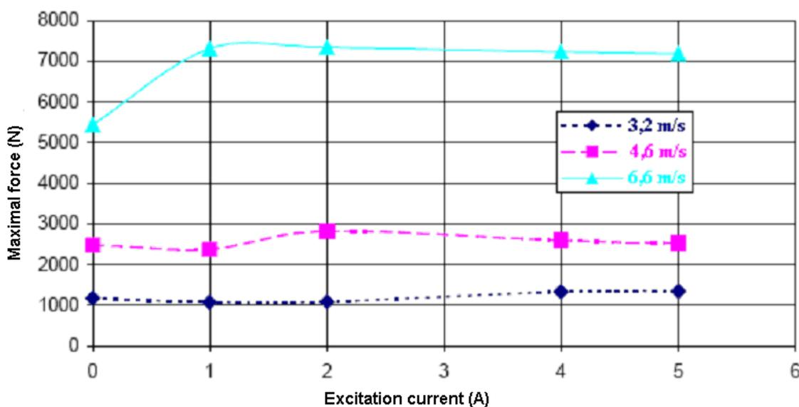
Fig. 4. Maximal force transmitted to the magnetorheological damper as a function of excitation current
