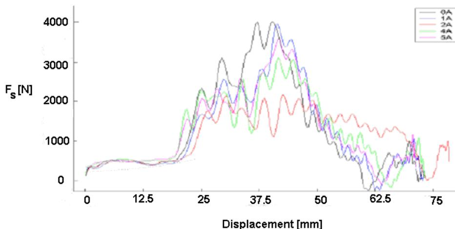
**Fig. 7. Transmitted force from the damper to the base, as a function of displacement**
