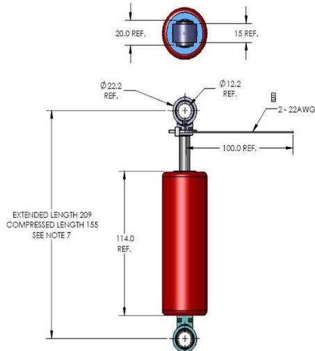
Fig. 2. Magnetorheological damper
