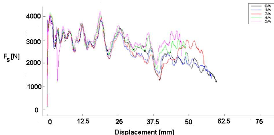
**Fig. 9. Transmitted force from the damper to the base, as a function of displacement**
