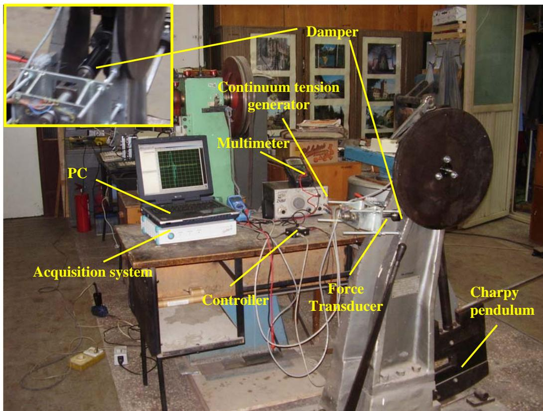
**Fig. 5. Experimental test bench**
