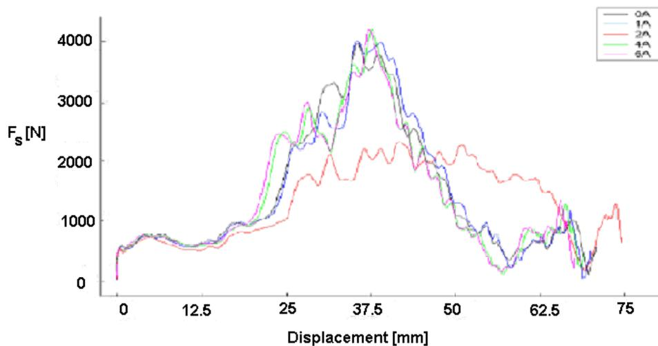
**Fig. 8. Transmitted force from the damper to the base, as a function of displacement**
