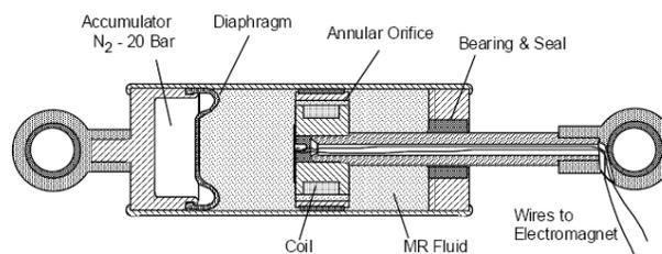
Fig. 3. Cross section of RD-1005-3
