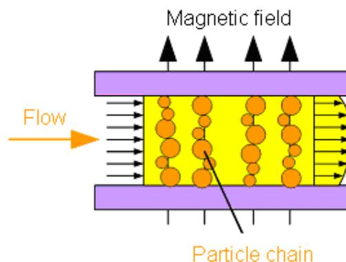
*Fig. 1. Work of magnetorheological fluid by flow control.*
